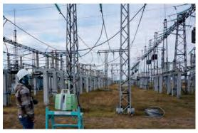
▲ Figure 1, Laser scanning of the power substation.
